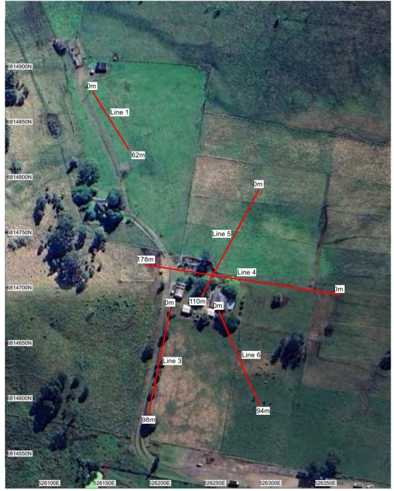
Figure 1: The survey area and locations of the acquired SR lines.
